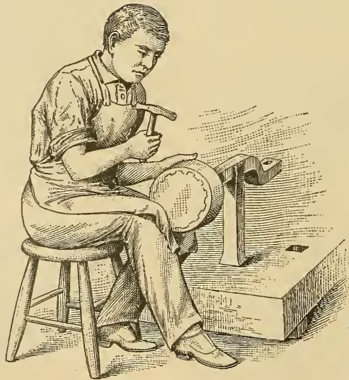
Fig. 107.—Planishing Tea-Kettle Side.
